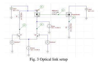
The driver circuit provides 50mA bias current and modulation current of 40mA. The transistor Q1 & Q2 is biased with Vpulse 1 and Vpulse2 of 2.5V. The dc current source Idc2 draws laser bias current of 50mA. The transient analysis for the circuit is performed for 10ns. The laser diode current is switching between 50-90mA as shown in fig. 4.
